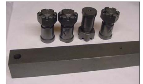
Crosshead Pins & Guides
